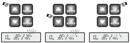
**SWITCHING ON THE DOMESTIC HOT WATER PUMP.** - Press the key  $(\bigtriangledown)$ , the domestic hot water temperature is flashing on the display. Press and hold the key  $(\bigtriangledown)$ , release it when two horizontal lines appear on the display instead of the temperature. Confirm by pressing the key (ENTER)
