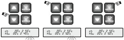
**SUMMER MODE** - Press the key  $(\triangle)$ , the central heating temperature is flashing on the display. Press and hold the key  $(\bigtriangledown)$ , release it when two horizontal lines appear on the display instead of the temperature. Confirm by pressing the key (ENTER)
